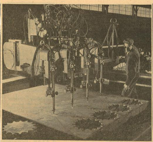
NEW FLAME CUTTER—Harry Zechmeister operates a new electronic tracer torch burning equipment that reduces scrap loss and eliminates excessive handling and machining of steel shapes. In the above operation he is cutting gear sprockets in multiple units from one inch
